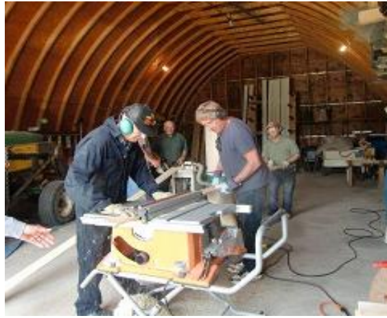
Bill Chimboryk, Norm Dyck and Bill Rafoss using table saw to cut siding to proper width
